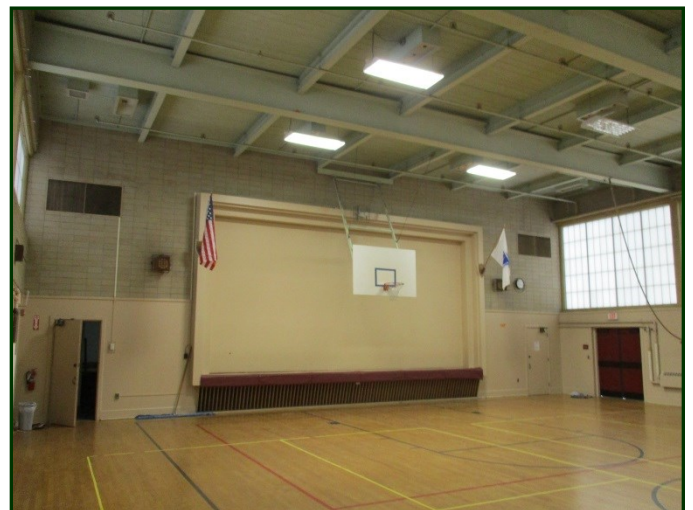
Photo #72: Gymnasium with maple flooring, CMU walls and exposed underside of structure above
